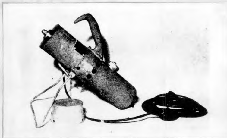
A mist machine which produces droplets by means of centrifugal force. The formulation is emitted from between two closely approximated whirling discs. From: Correspondence Course in Pest Control Technology, by Lee C. Truman (1961).
