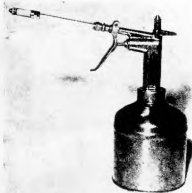
Figure 240. A small, hand-operated, piston type, hydraulic sprayer. (Photo by Hazel-tine.)
