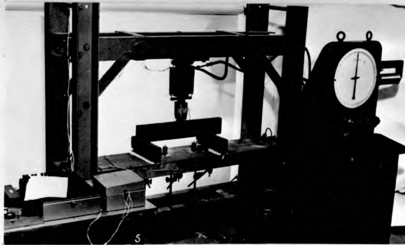
FIG. 43. GENERAL VIEW OF THE STRIP BEAM TESTING RIG
