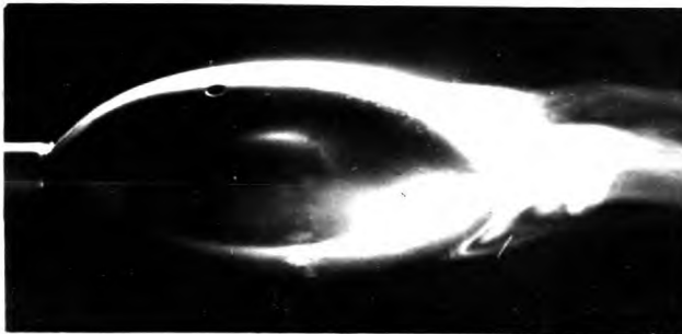
(iii) \phi_{\max} \simeq 40^\circ SEPARATED REGION FURTHER DECREASED
