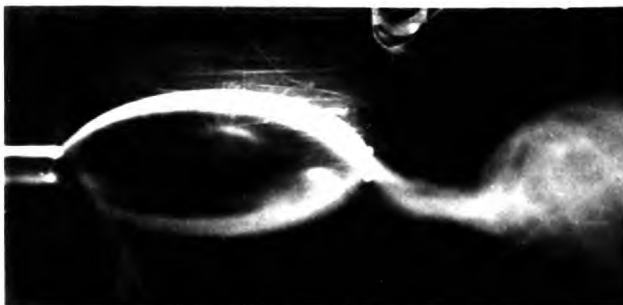
(iv) \phi_{\max} \simeq 60^\circ ATTACHED FLOW FOLLOWED BY VORTEX BURST
