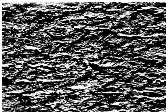
Figure 5.6. Wavy slip lines on the (100) plane after 30% tensile strain at 353 o K. x 200
