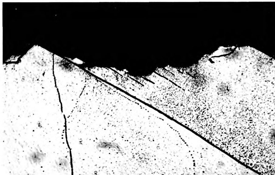
Figure 5.28. Fracture propagated along a twin boundary in a crystal deformed at 77^{\circ}\text{K} in the \langle 100 \rangle direction. Surface etched with etchant b). \times 200 .
