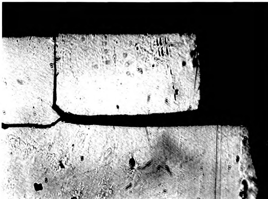
Figure 5.19. The appearance of the slip lines and fracture profile on a \{100\} plane of a crystal deformed in the \langle 100 \rangle direction at 195^{\circ}\text{K} . \times 200 .
