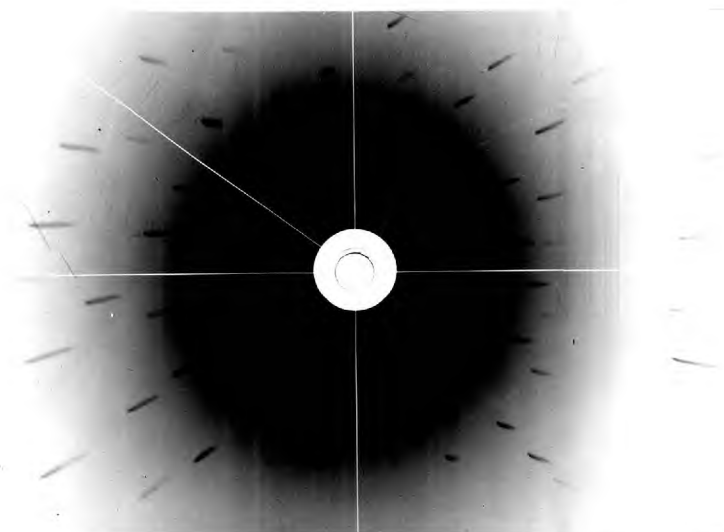
Figure 5.13. Asterism of the Laue spots for a crystal deformed at 77°K. The [100] direction is almost perpendicular to the plane of the photograph.
