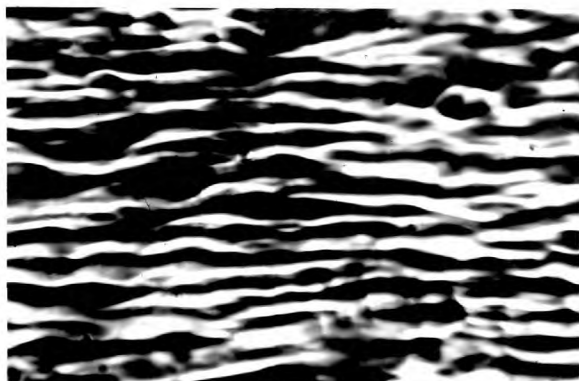
Figure 5.5. Wavy slip lines on the (100) plane after 25% compressive strain at 293 o K. x 140.
