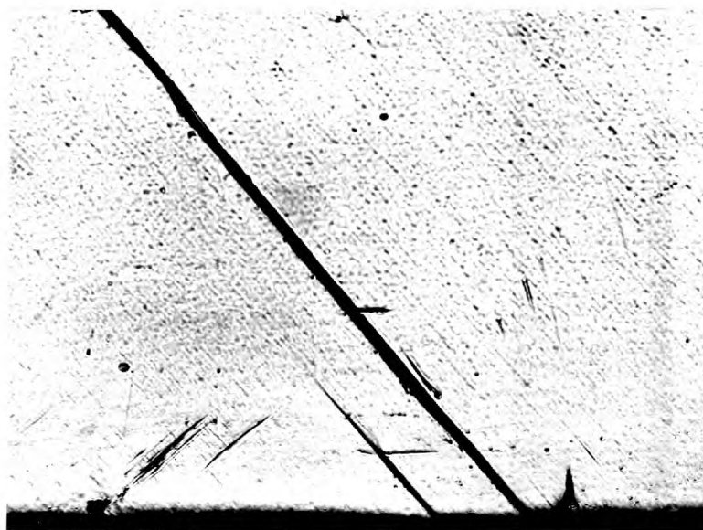
Figure 5.20. Slip lines on a \{100\} plane of a crystal deformed in the \langle 100 \rangle direction at 353^{\circ}\text{K} . \times 200 .
