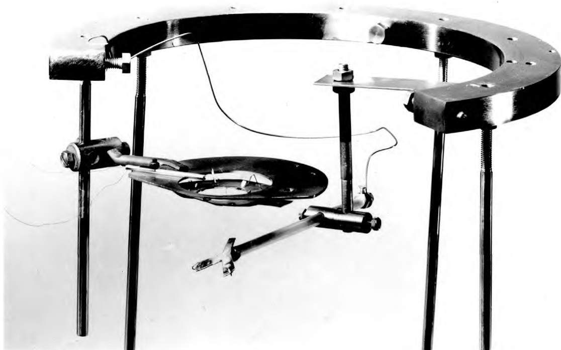
FIG. 3.8. TARGET AND SUBSTRATE HOLDERS FOR THE EPITAXIAL DEPOSITION OF Si
