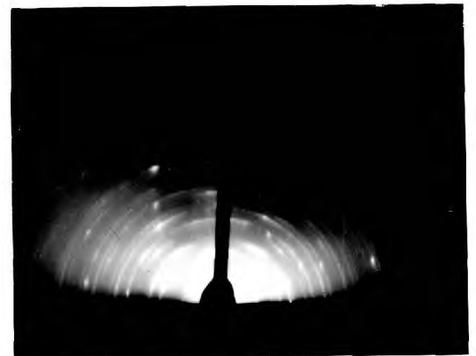
Polycrystalline layer grown at 700°C
