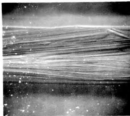
FIG. 4.15. POLYCRYSTALLINE Si TARGET AFTER CHEMICALLY ETCHING FOR FEW MINUTES ONLY
