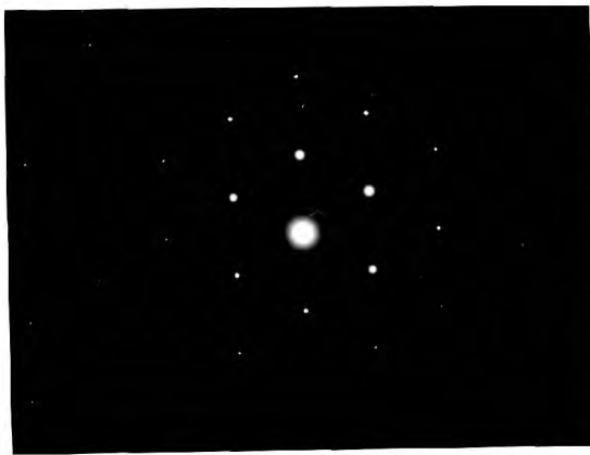
(111) pattern Single crystal layer grown at 840°C (110) pattern
