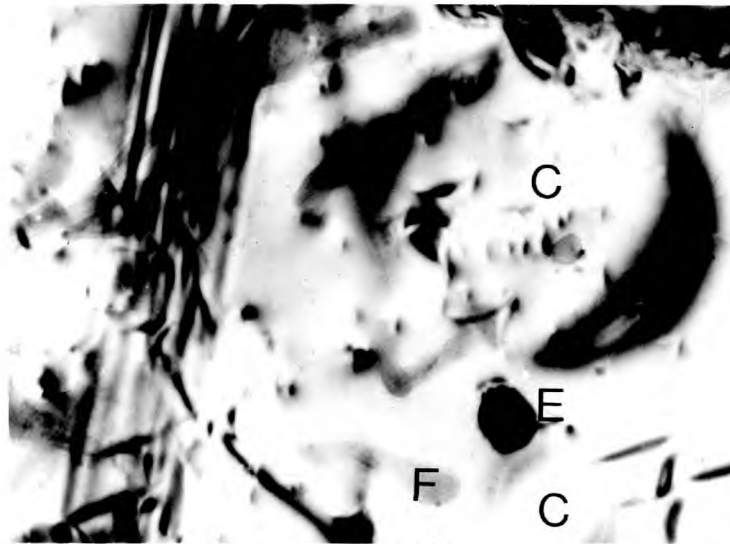
FIG. 4.7. TRANSMISSION ELECTRON MICROGRAPHS OF LAYER DEPOSITED AT 990°C ONTO SUBSTRATE AT EARTH POTENTIAL WITH NO SHUTTER BETWEEN TARGET AND SUBSTRATE (ION BEAM 12keV 4.4mA)
