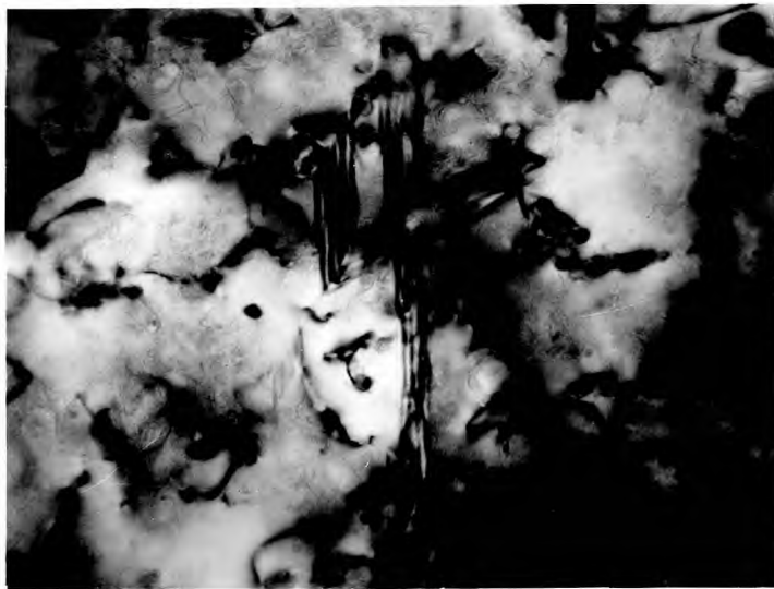
(i) Ion beam 12keV 5.5mA, temperature about 920°C
