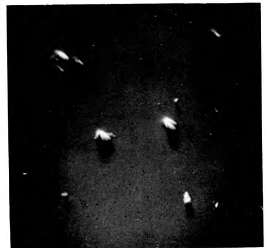
FIG. 4.13. CONICAL PROTRUSIONS FORMED ON "(111)" Si SURFACES BY ION BOMBARDMENT
