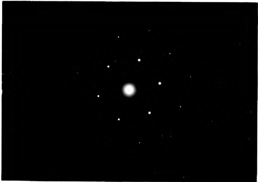
(b) Diffraction from region of thickness about 2000 Å
