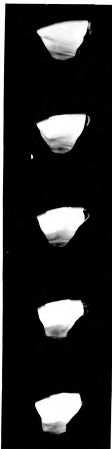
Figure 26: The 'CO Boil' in an Iron-Carbon Alloy Drop. (Film No.8 taken at 1000 frames/second)
