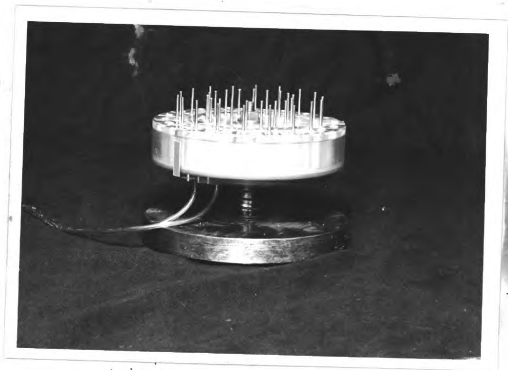
Fig. A.1.3 Rotary Pressure Switch.
