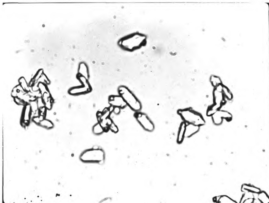
Figure 11. Sodium calcium hydrosilicate crystals obtained from the treatment of (a) Quartz, 1000X; and (b) Muscovite, 800X, in 500 g/l NaOH solutions at 280°C for 1 hour.
