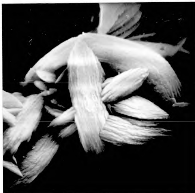
The interpenetrating twins of K-G showing growth steps magnification 6000X
