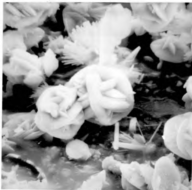
The cocrystallization of K-G with K-M (radiating rods) magnification 3000X
