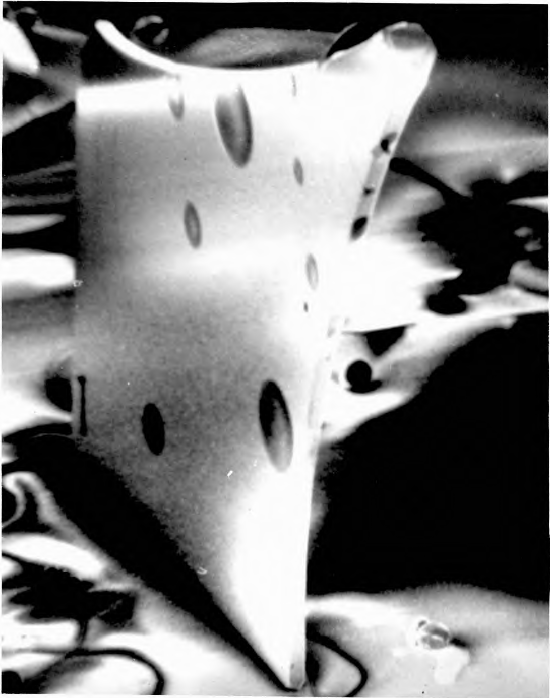
Fig. (3.10) Scanning Electron Micrograph of Kite Shaped Platelet stood on edge. (This platelet is the one arrowed in Fig. (3.5.c))
