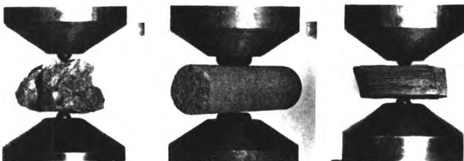
Figure 46: Three types of point load best suited for practical strength classification.
