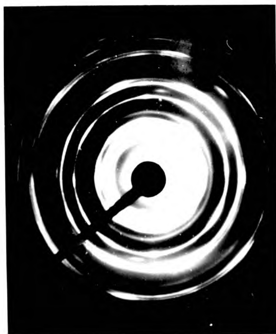
Figure 5.3 Electron micrographs ( \times 100000 ) and diffraction patterns of films grown on (a) NaF and (b) LiF at various temperatures
