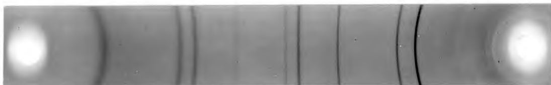
Film 2. Homogeneously deposited palladium.
