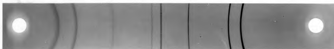
Film 1. Nickel deposited from solution.
