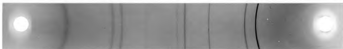
Film 2. Homogeneously deposited palladium.
