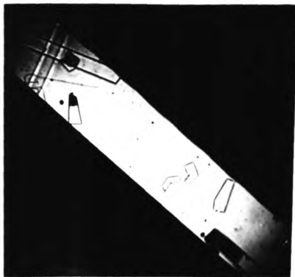
Figure 3.5(b) Ribbon crystal viewed between crossed polaroids (magnification X50)
