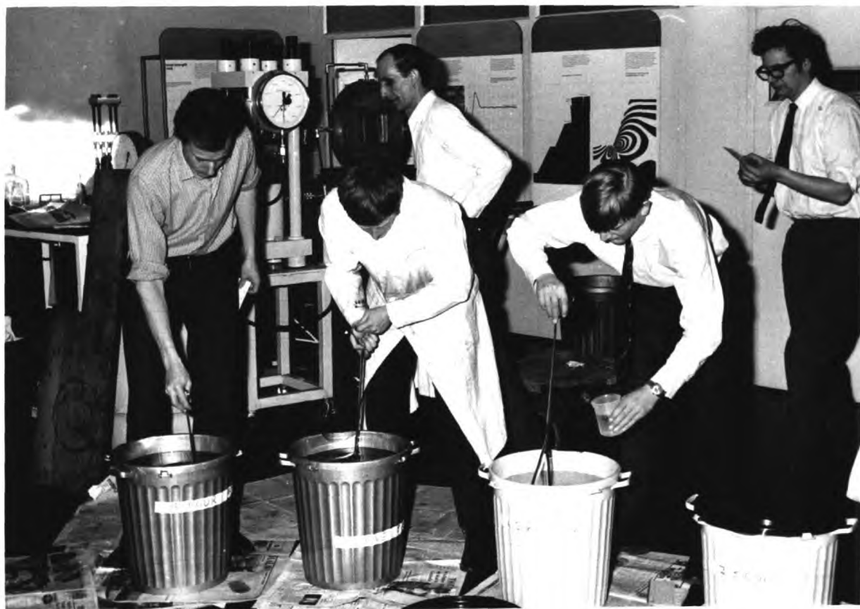
STIRRING THE CATALYST INTO THE RUBBER. Four of the twelve dustbins are shown.
