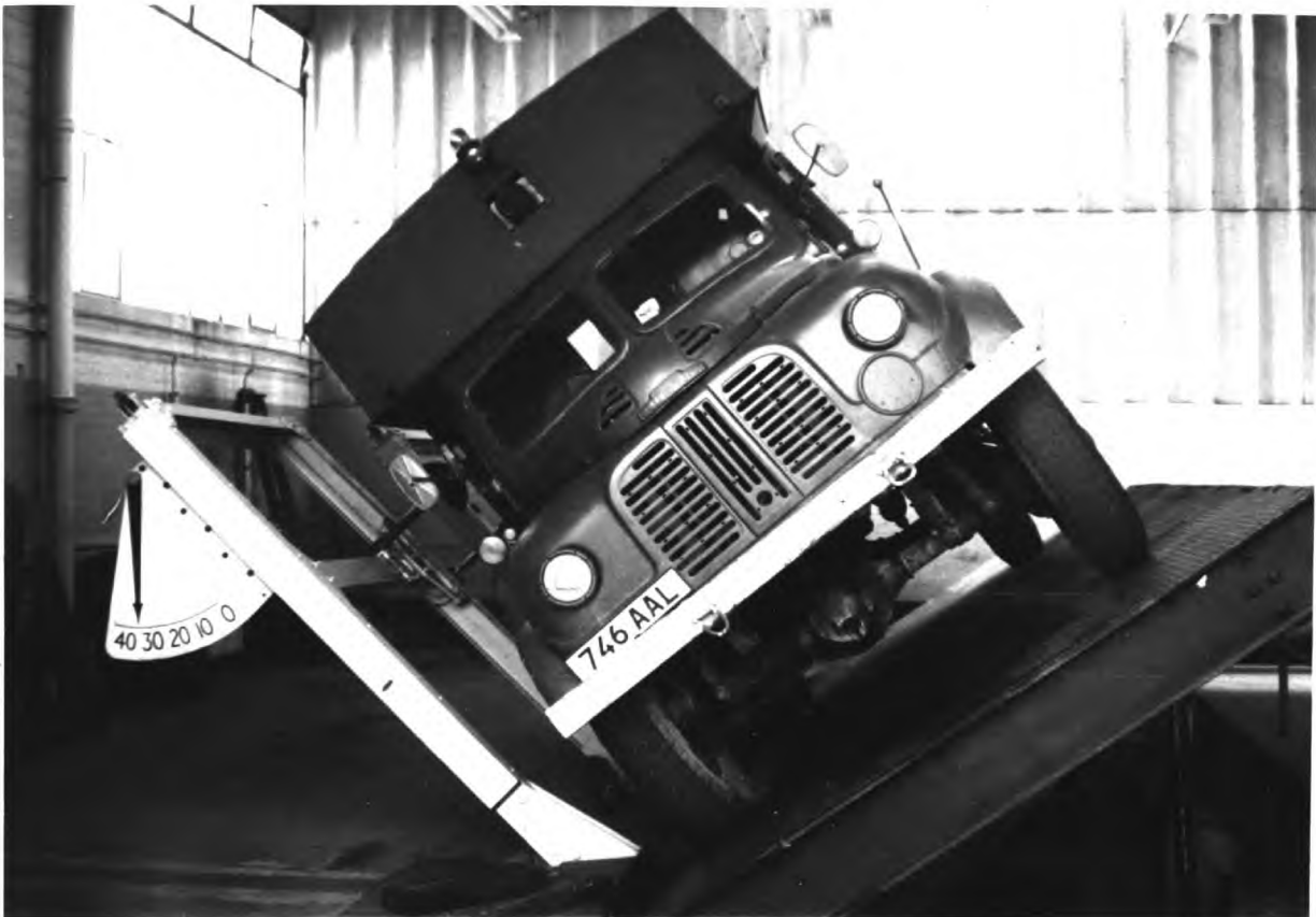
FIG. 8: TILTING TEST PERFORMED ON THE TRUCK: the photograph shows it on the point of toppling.
