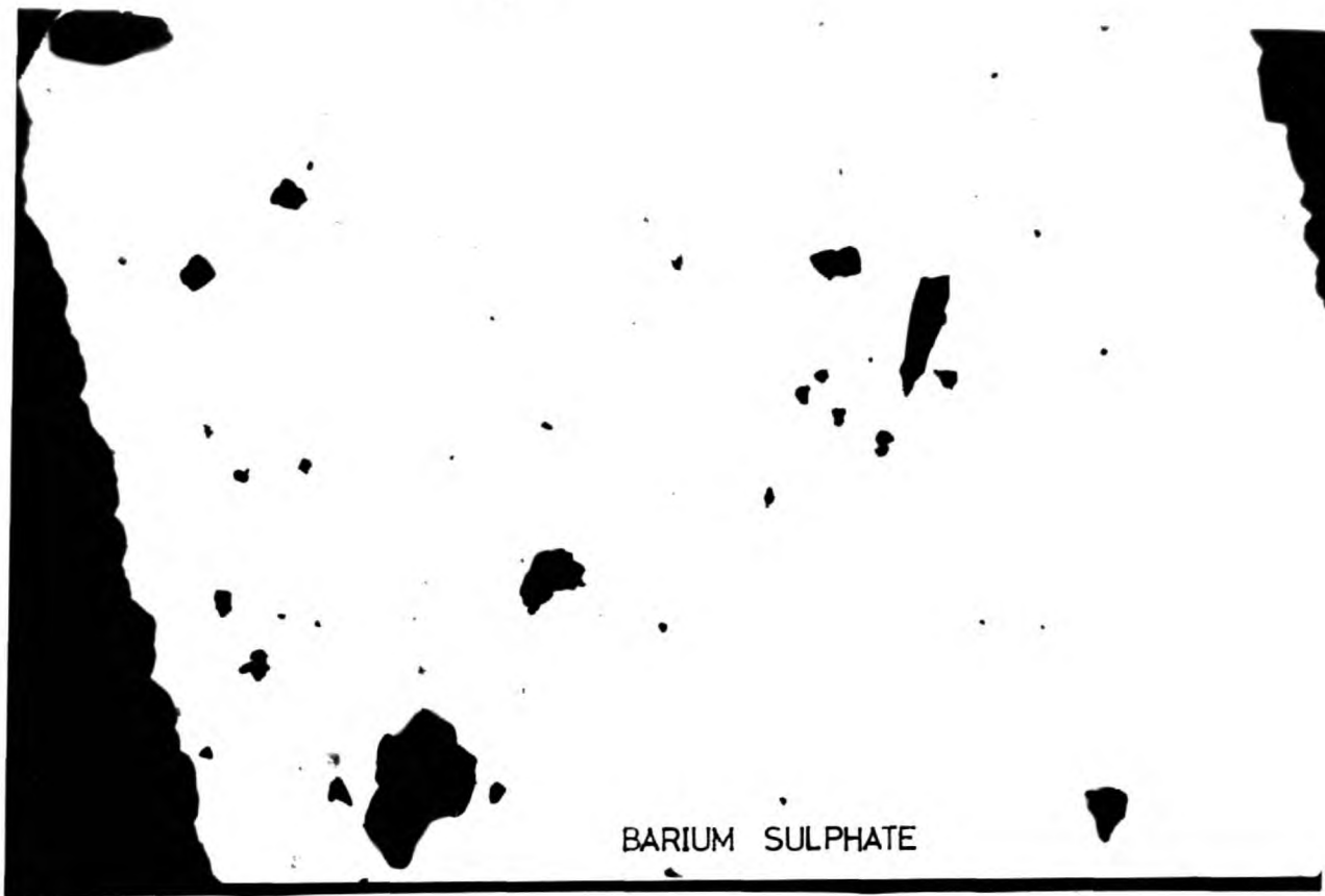
FIG. 8A ELECTRON MICROGRAPH OF PIGMENTS 1.8 mm = 1 micron
