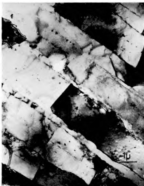
FIG. 16. Longitudinal section of an extruded rod manufactured from powder A. Initial billet temperature 300^{\circ}\text{C} , extrusion ratio 30:1.
