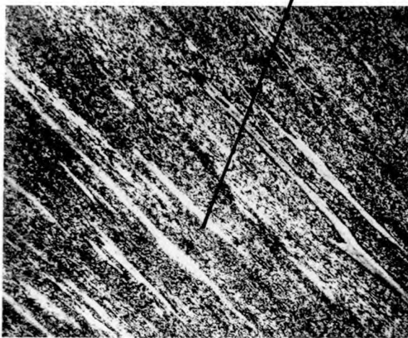
PLATE 5 6 Longitudinal section of a partially extruded billet. Macrophoto, etched. Photomicrographs, etched X 64
