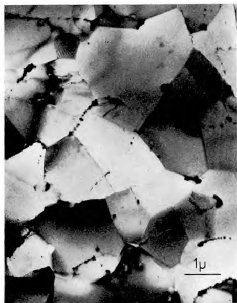
FIG. 18. Transverse section of an extruded rod manufactured from powder B. Initial billet temperature 300°C, extrusion ratio 30:1.
