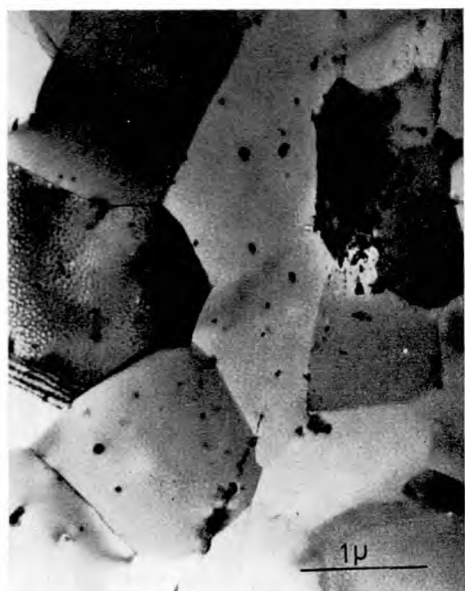
FIG. 20. Transverse section of an extruded rod manufactured from powder B. Initial billet temperature 150°C, extrusion ratio 30:1.
