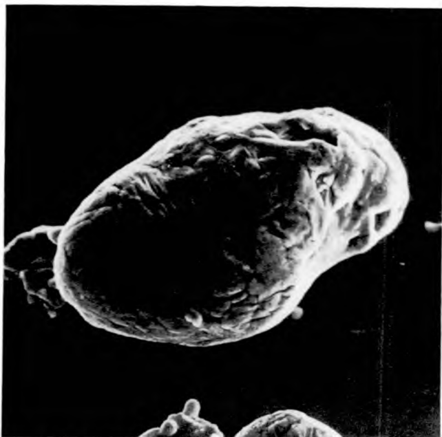
FIG. 14. An aluminium particle of powder A. \times 1360 .
