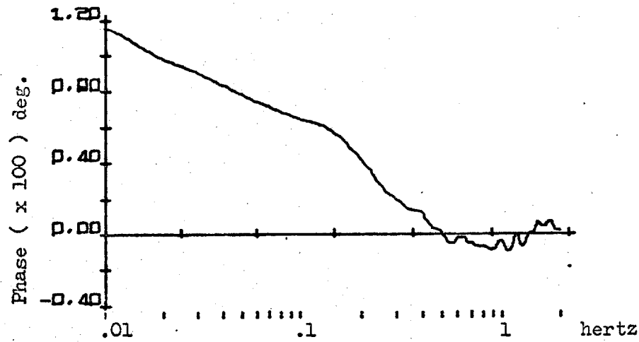
Figure IV.9 b. Frequency spectra of the error function, as derived from averaged step responses.
