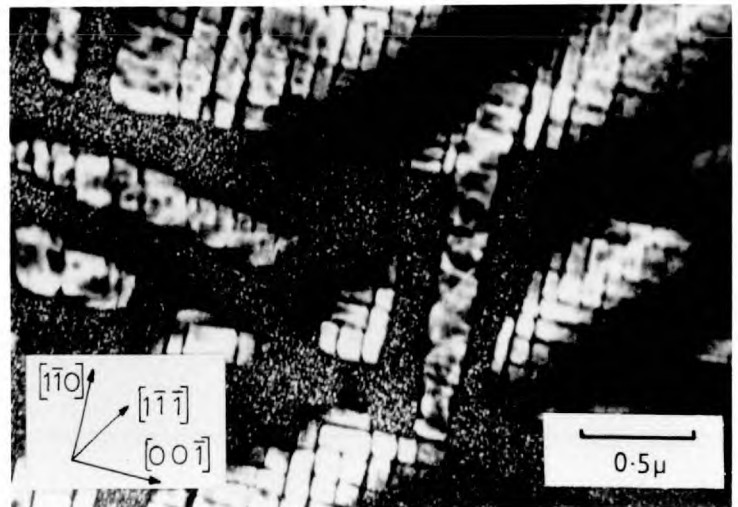
Fig.5:6c ALLOY 20T 1020°C 1hr - 850°C ½hr - W.Q. More pronounced {110} interphase boundaries.
