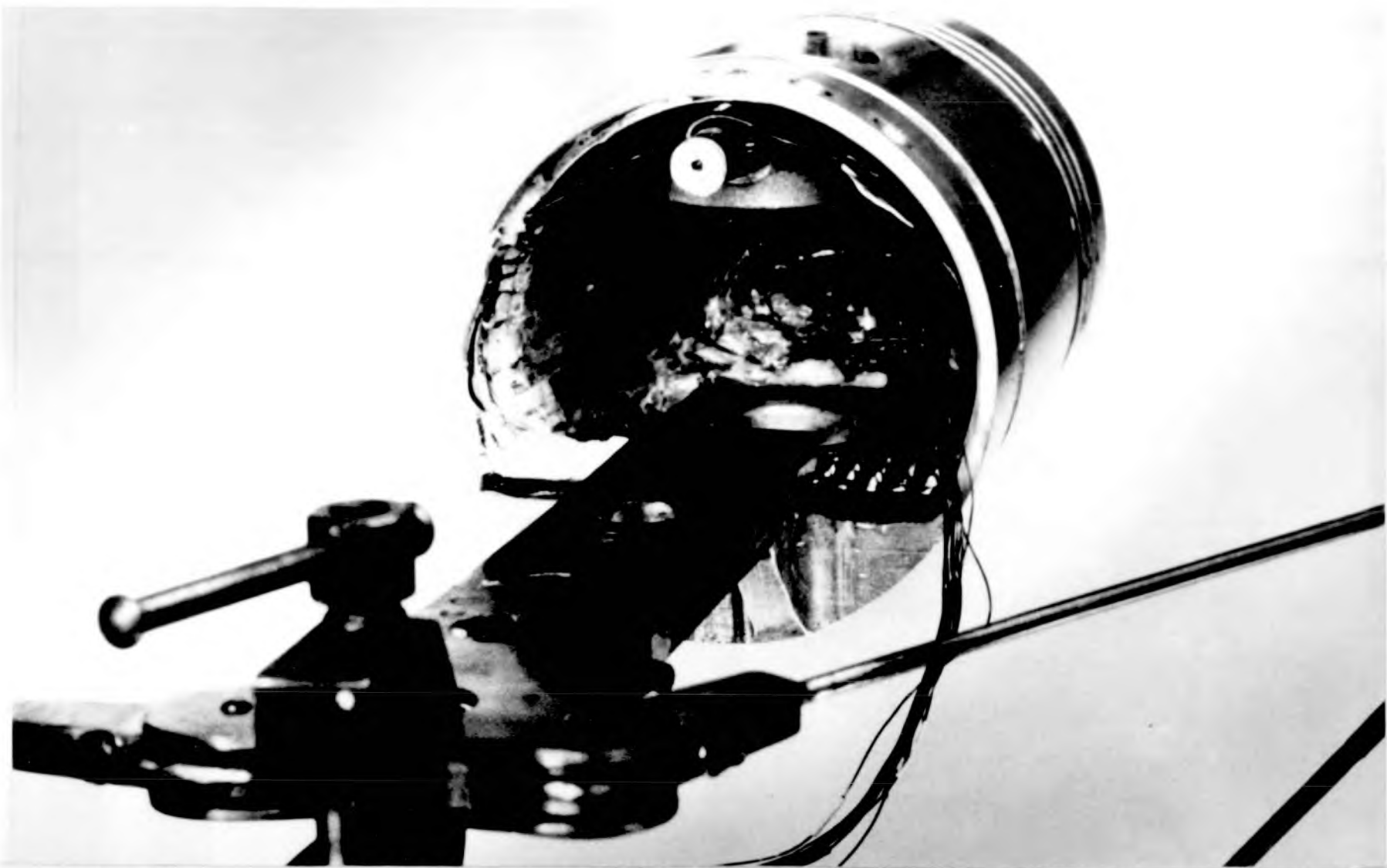
PLATE 10 - PARTIALLY WIRED PISTON WITH FLEXIBLE CIRCUIT AND SOME WIRING IN POSITION
