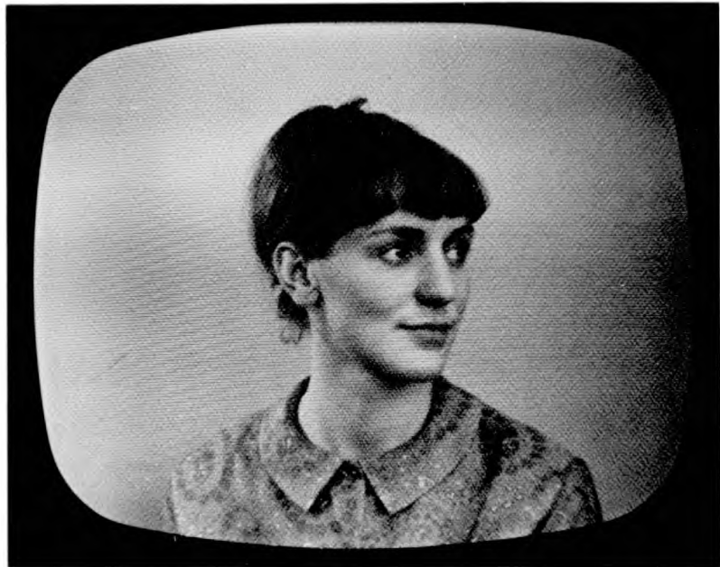
(b) "Rectangular" spectrum rising to 3 MHz horizontally and '1.5 MHz' vertically.
