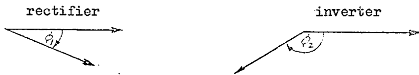
Fig. 2.3 Phasor relationship of converter voltage and current.
