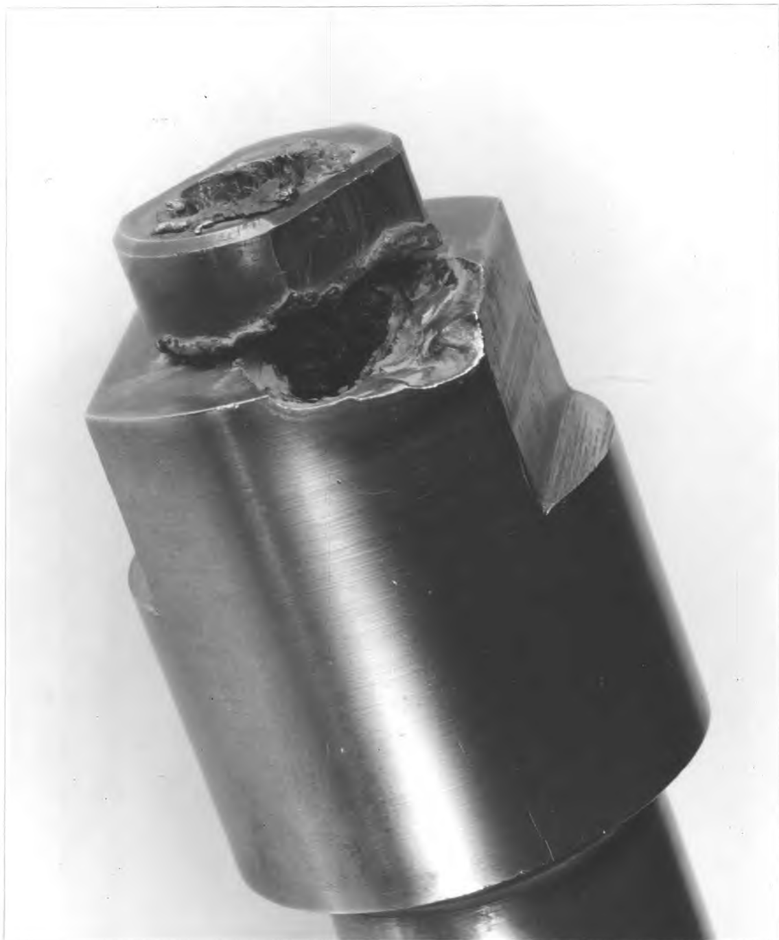
Plate No. 2. A photograph of the burnt away electrode ( \times 2 ).
