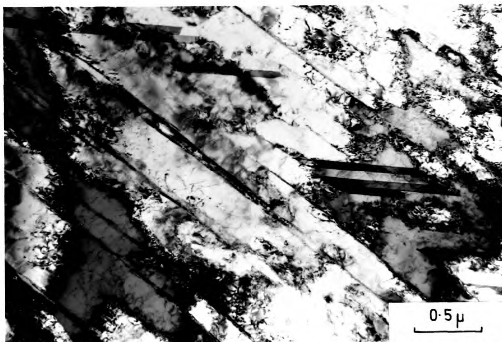
FIG. 4.33. Alloy B. Twins in austenite after heating the cold rolled structure for 1 minute at 775°C.
