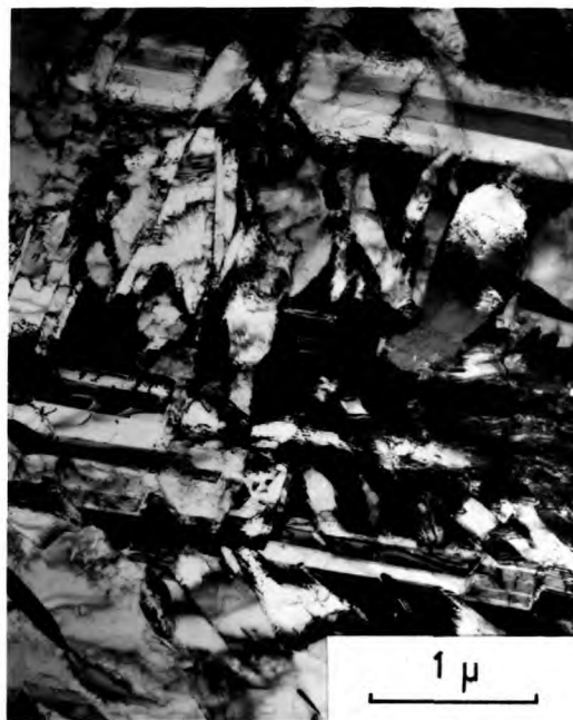
FIG. 4.11. Alloy A. Heated for 2 minutes at 550^{\circ}\text{C} after quenching to -196^{\circ}\text{C} for 15 minutes.
