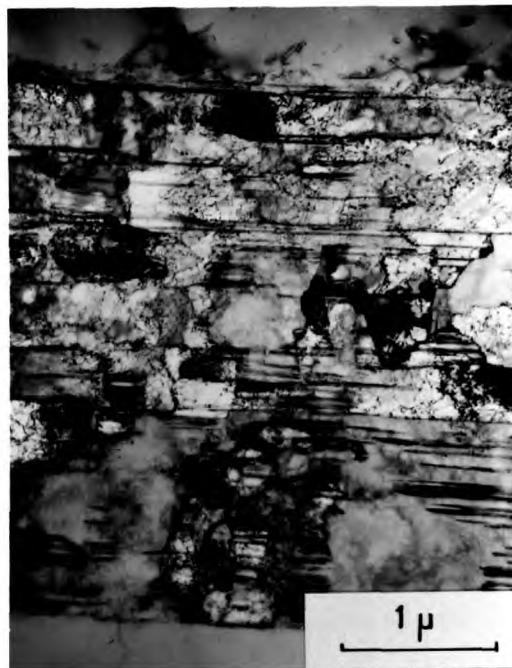
FIG. 4.9. Alloy A. Reversed austenite bounded by retained austenite; treated as in FIG. 4.8.
