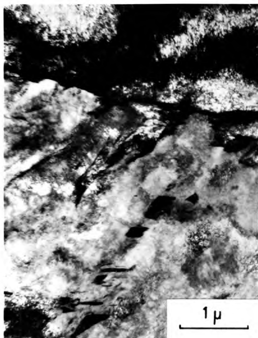
FIG. 4.55. Alloy B. Solution treated and aged at 700^{\circ}\text{C} for 310 hours.
