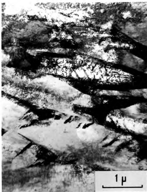
FIG. 4.53. Alloy B. Solution treated and aged at 650^{\circ}\text{C} for 1 hour.
