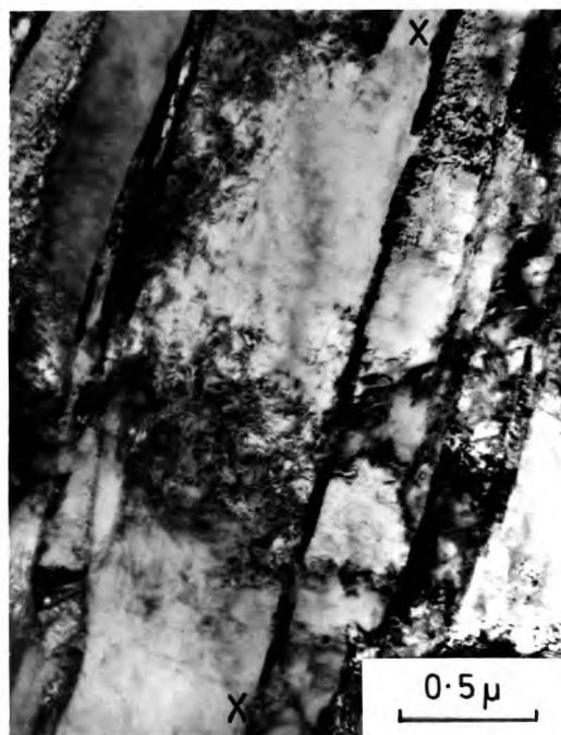
FIG. 4.56. Alloy B. Solution treated and aged at 700^{\circ}\text{C} for 310 hours.
