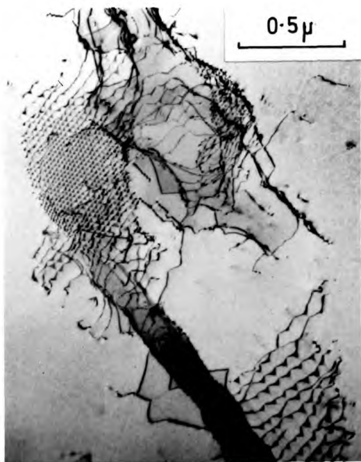
FIG. 4.45. Alloy A. Reversed austenite annealed for 5 hours at 850°C.
