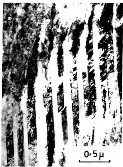
FIG. 4.27. Alloy A. Cold worked structure heated for 2 minutes at 600°C, showing twins in austenite.
