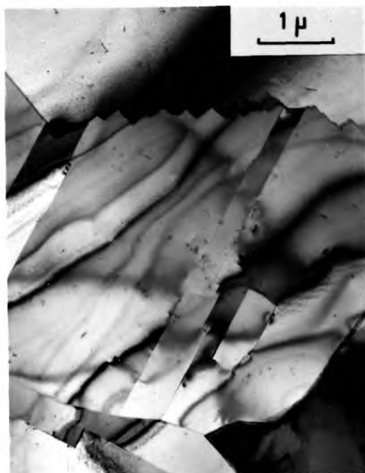
FIG. 4.49. Alloy A. Cold worked, reversed at 600°C for 2 minutes and annealed for 2 minutes at 850°C.
