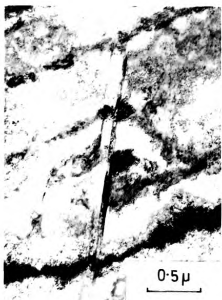
FIG. 4.28. Alloy A. Cold worked structure heated for 2 minutes at 525°C.
