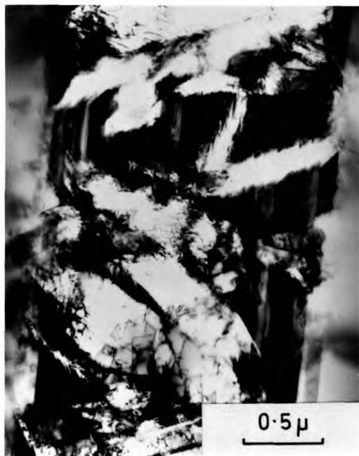
FIG. 4.10. Alloy A. Heated for 2 minutes at 525^{\circ}\text{C} after quenching to -196^{\circ}\text{C} for 15 minutes.
