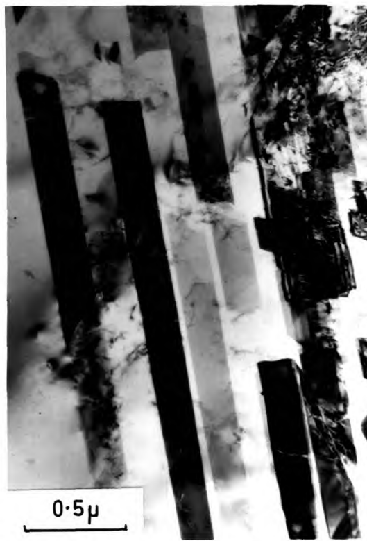
FIG. 4.14. Treated as for FIG. 4.13. showing clearly twins in what was originally a martensitic region.
