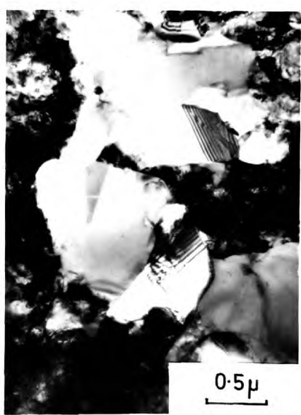
FIG. 4.29. Alloy A. Cold worked structure heated for 2 minutes at 555°C; recrystallised grains.
