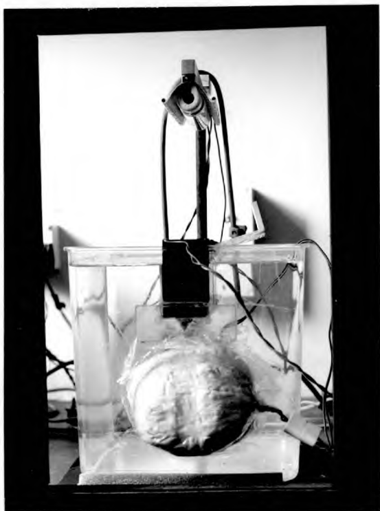
Fig. 8 d: B II in tank. Note overhead light, and buzzer (padded attachment to tank). Dark screen removed to show apparatus.
