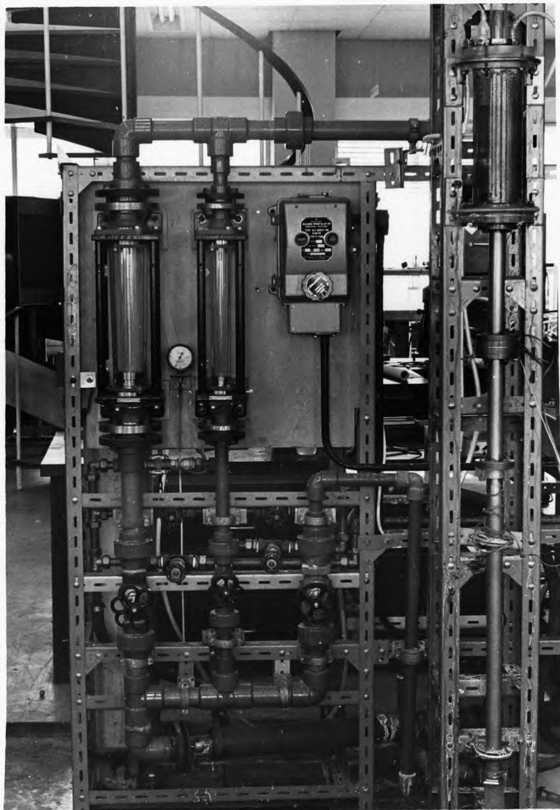
Fig. 7.3-2 The apparatus for mass-transfer experiments
