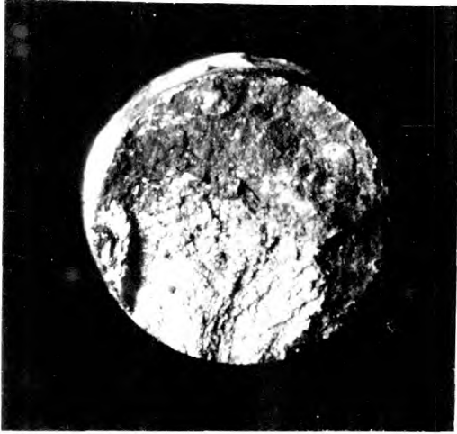
EXAMPLES OF STIRRUP FATIGUE FRACTURES
