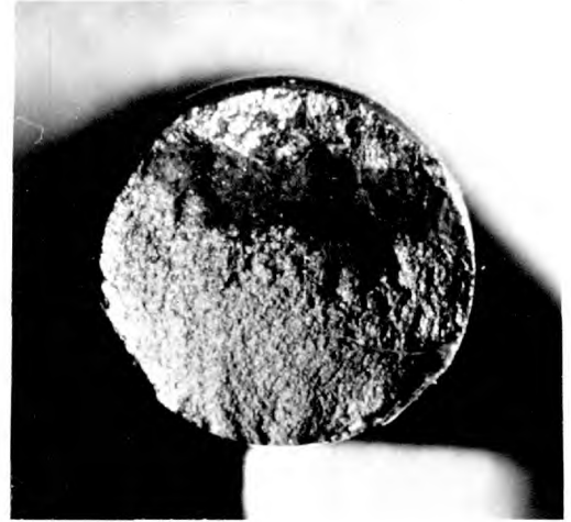
EXAMPLES OF STIRRUP FATIGUE FRACTURES
