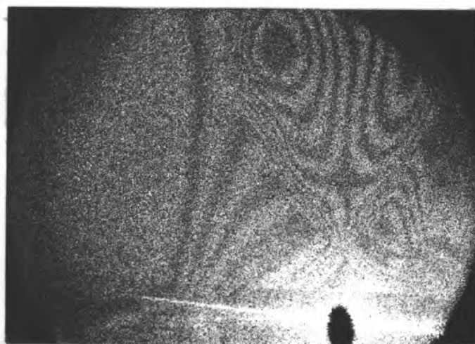
Fig (6.14) (a) & (b) Spatially resolved flame interferograms (c) Integrated interferogram obtained by increasing the depth of field for viewing the reconstructed images of the hologram.
