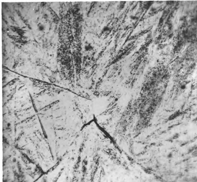
Fig.2.2. Effect of 0.2% plastic strain on formation of martensite in austenite. Dark regions are 'ghost' structure. X600
