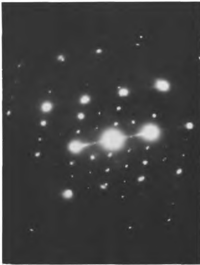
Fig. 3. 32a. S.A.D. from tempered S.T.A. martensite in fig. 3. 32b.
