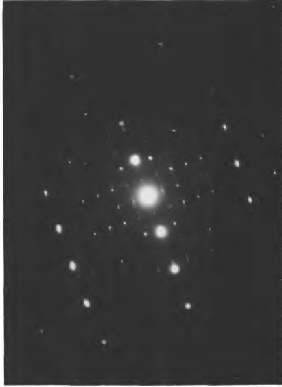
Fig. 3.33a. S.A.D. from tempered conventional martensite in fig. 3.33b.
