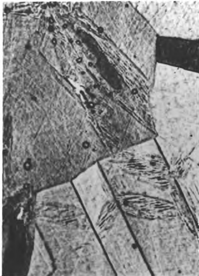
Fig. 3.9a. HP1 alloy. 'Ghost' structure of martensite in austen- ite X800
