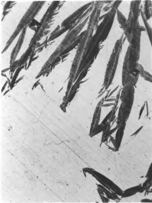
Fig. 3.1a. Conventional martensite and austenite structure X540
