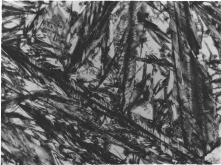
Fig. 3.29a. Carbide precipitation along the twin boundaries X650
