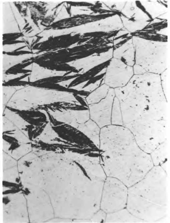
Fig. 3.1b. Structure after austenitizing at 650°C for one minute X540
