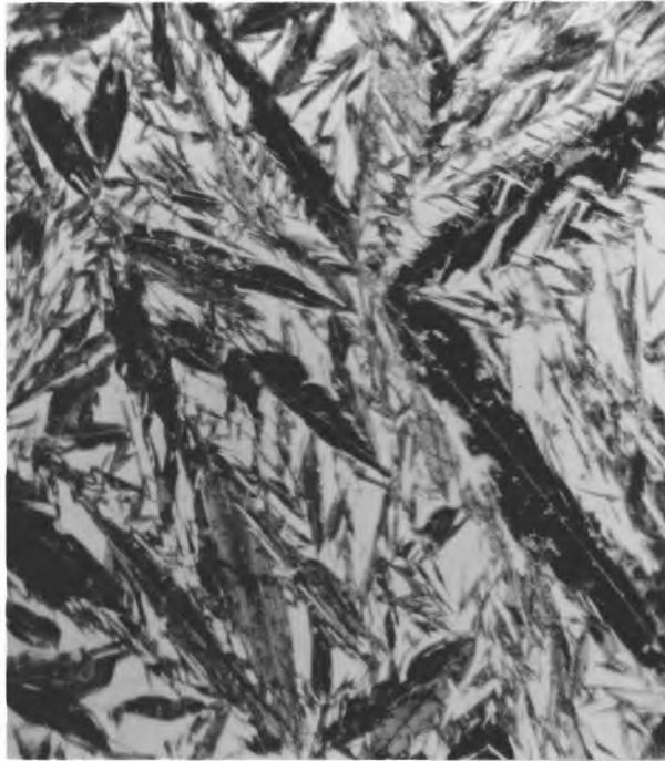
Fig. 3.21a. Conventional martensite X550
