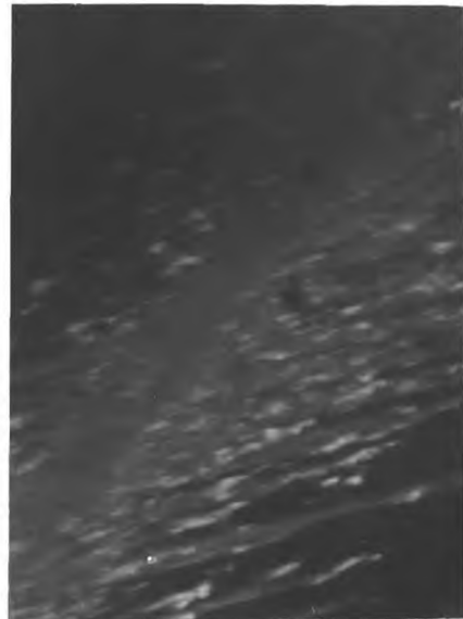
Fig. 3.29c. Dark field transmission using carbide reflection showing precipitation along the original twins X20,000
