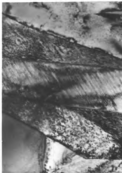
Fig. 3.1c. Twinned and un-twinned nature of martensite X40,000
