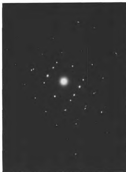
Fig. 3.13b. S.A.D. of fig. 3.13a. foil orientation \{110\}
