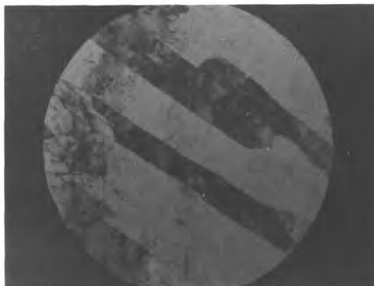
Fig. 3.13a. Fragments of S.T.A. austenite are seen. Note irregular nature of the boundaries X40,000
