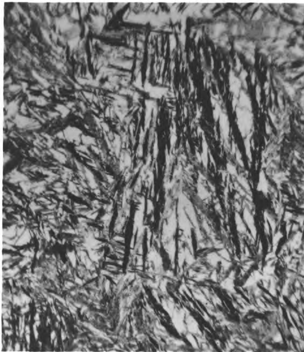
Fig. 3.21b. S.T.A. martensite structure, showing narrower mar- tensite plates (c. f. fig. 3.21a) X550
