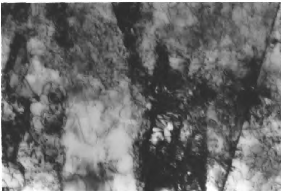
Fig. 3.14b. Fe-Ni-C (INN1) alloy austenitized for 5 seconds at 650°C. showing high density of dislocations and sub-boundaries X80,000
