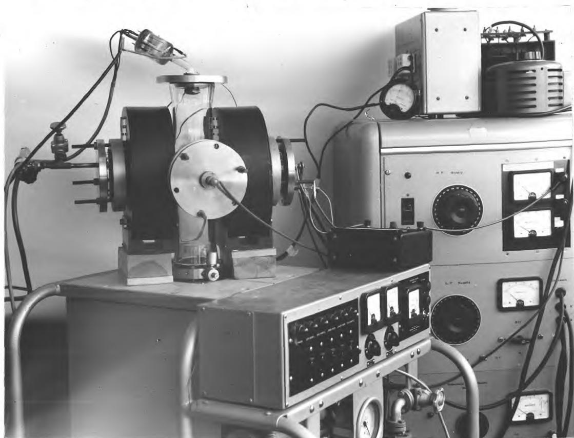
in Fig. 4.10. The electrodes and other inlets were introduced through the stainless steel closure flanges, the seals being made with Viton 'O'-rings or with a cold setting low volatile resin ("Torr-seal", manufactured by Varian Associates and recommended for vacuum work down to  $10^{-8}$  torr).
