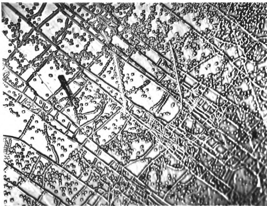
The dislocation arrangement in deformed crystal after completion of conductivity run Fig. 1.12c
