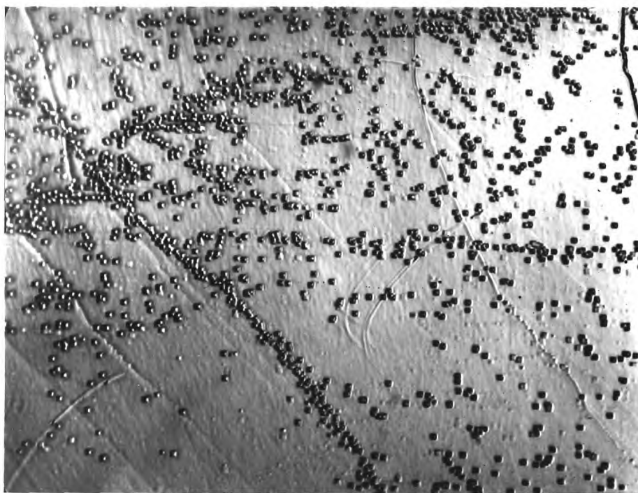
The dislocation arrangements in pure crystals of NaCl, annealed at 700°C and slowly cooled. Fig. 1.12a.
