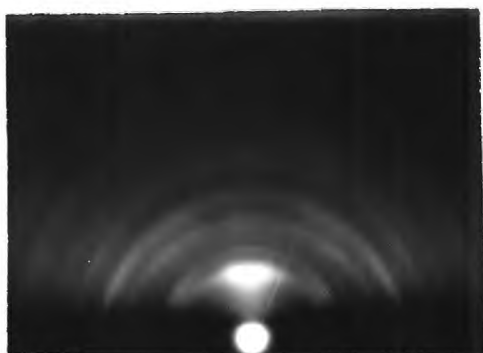
(c) Thickness = 2200A at i=0^\circ Pressure = 2 \times 10^{-7} torr Angle i = 0^\circ
