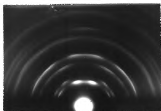
15b. Thickness = 2600Å at i=0^\circ Pressure = 5 \times 10^{-5} torr Angle i = 0^\circ
