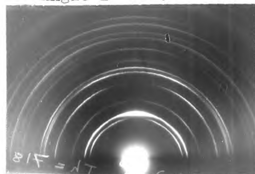
(e) Thickness = 718A at 71A/sec at i=0^\circ Pressure = 5 \times 10^{-3} torr Angle i = 0^\circ
