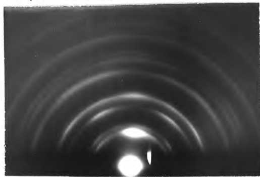
(e) Thickness = 1400A at i=0^\circ Pressure = 5 \times 10^{-6} torr Angle i = 45^\circ ← Vapour
