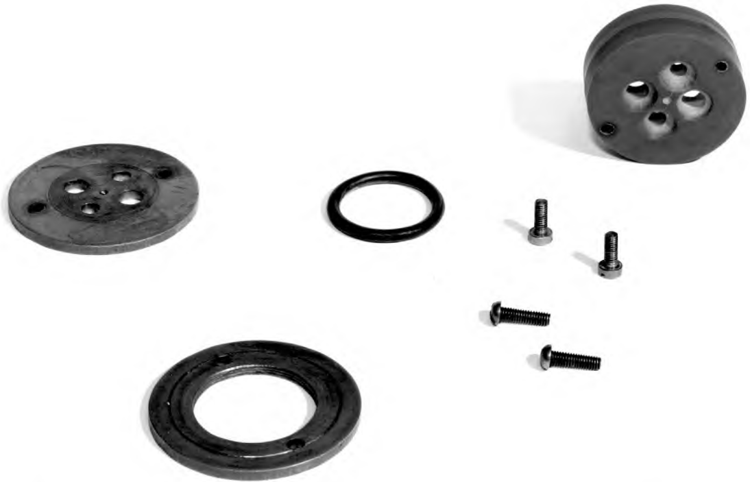
Fig. 17a Components: tufnol base, O-ring, brass ring and base plate.
