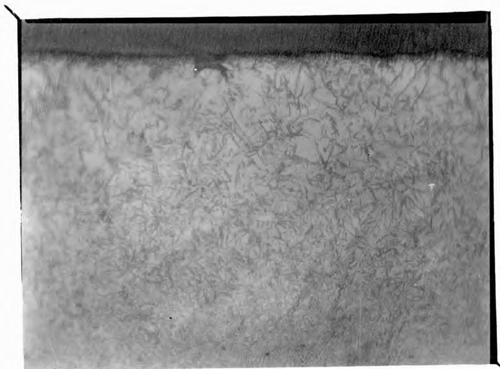
Fig. 67. Decrease in austenite content with increase in depth.
