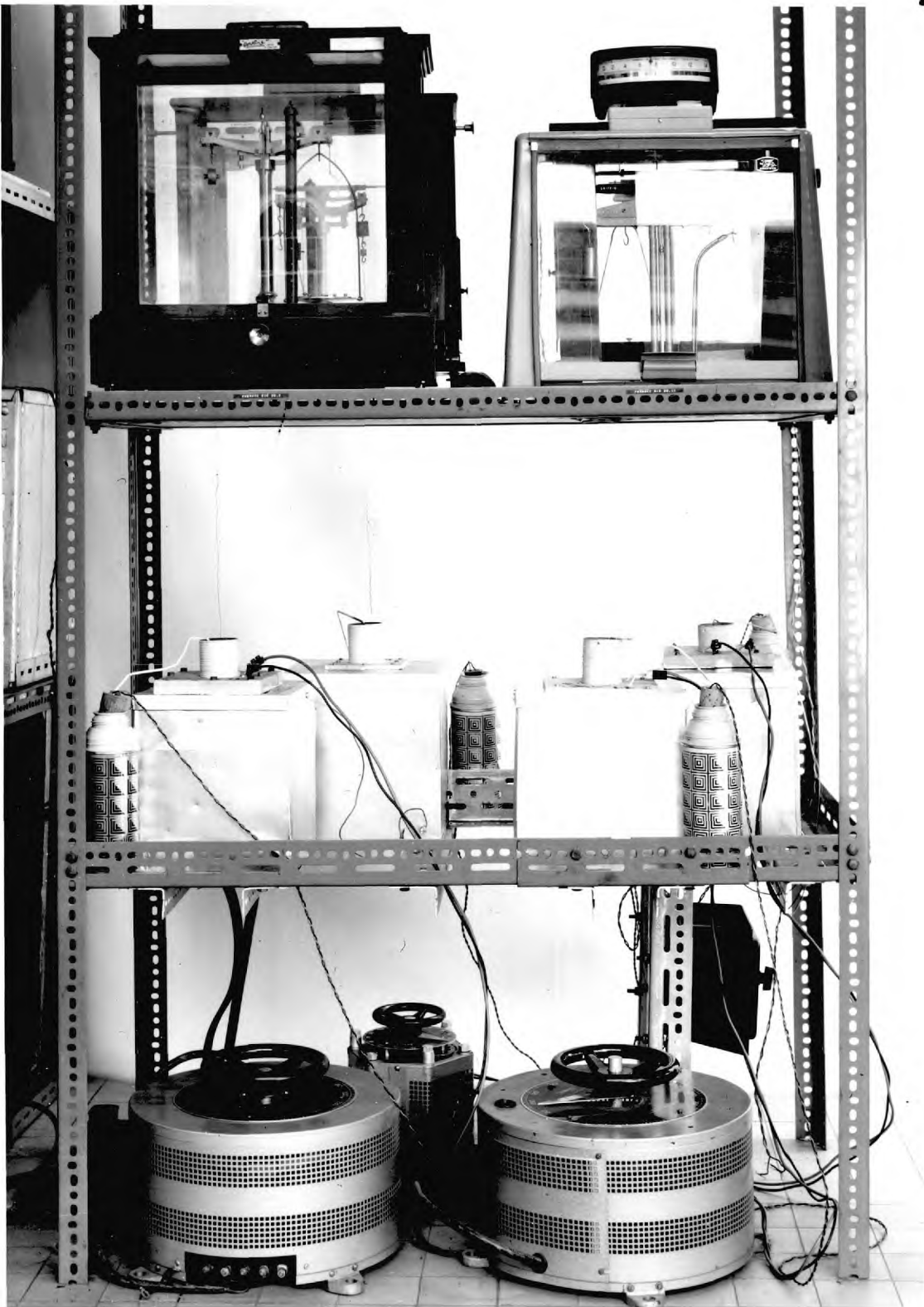
PLATE 2. ASSEMBLY OF FURNACES FOR CONTINUOUS WEIGHING
