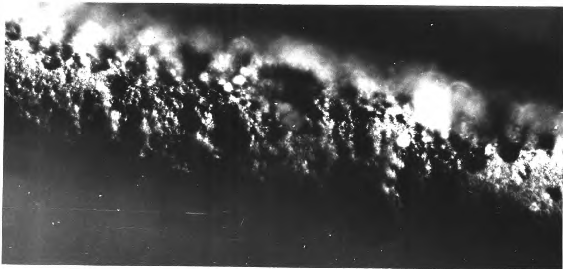
Photo 24. \text{UO}_3 treated filament No. 41; reacted in \text{O}_2 . x200
