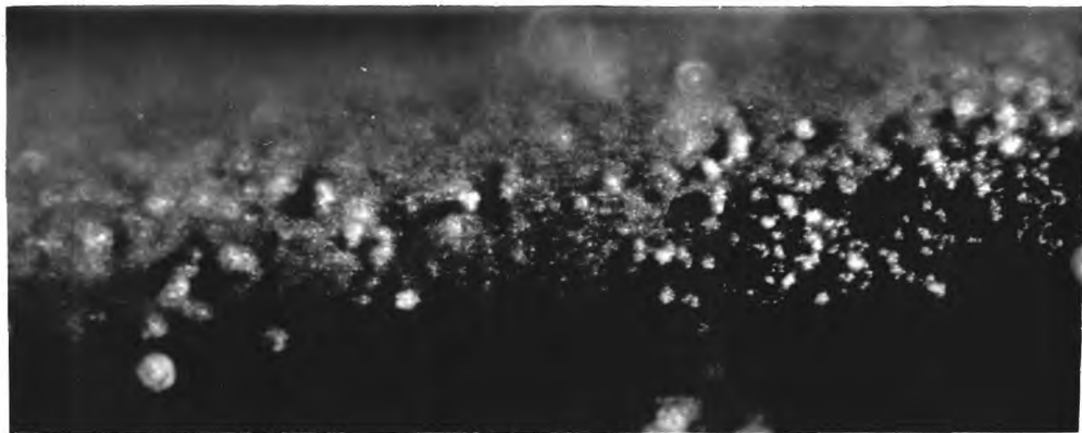
Photo 20. Molybdenum metal treated filament No.33. x200
