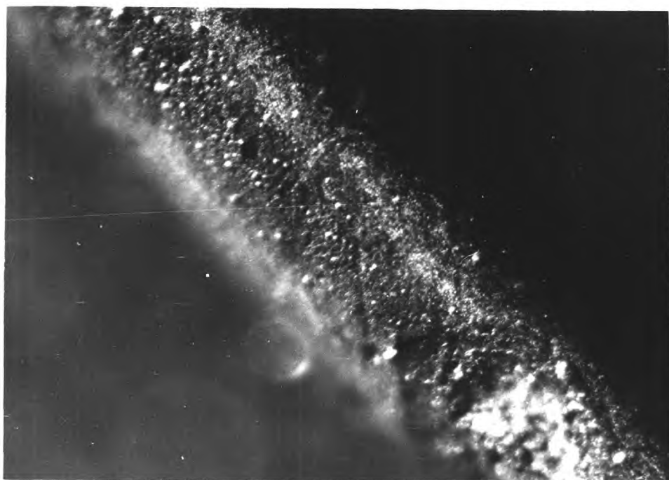
Photo 14. Sodium silicate treated filament No.40. x200
