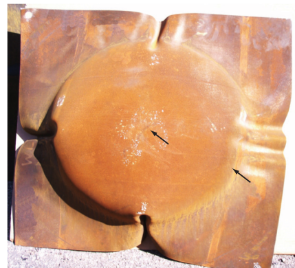
Figure 5: Deformed TWIP steel plate post blast testing. Arrows denote regions from which material was obtained for microstructure characterisation.
