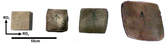
Fig. 1: Initial \beta annealed and as-rolled samples examined.
