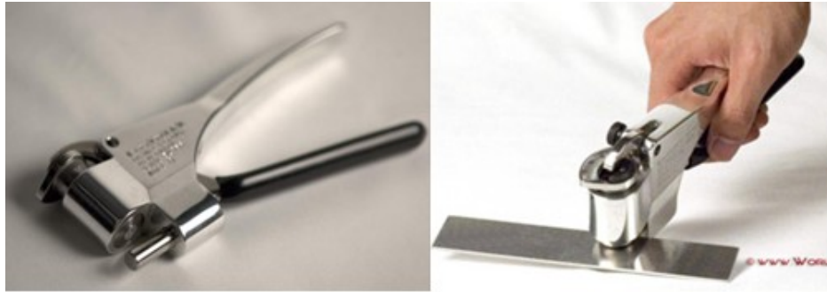
Fig. 3.3 Surface hardness measurements by Webster Hardness Gage
