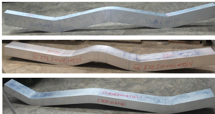
Fig. 3.25 Location of plastic hinges in deformed continuous beams (N50×95×10.5B5I, N120×70×10.5B5II and H95×50×10.5B5III)
