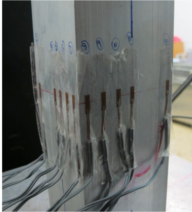
Fig. A.1.2 Specimen attached with strain gauges at one quarter of the cross-section at the mid-span
