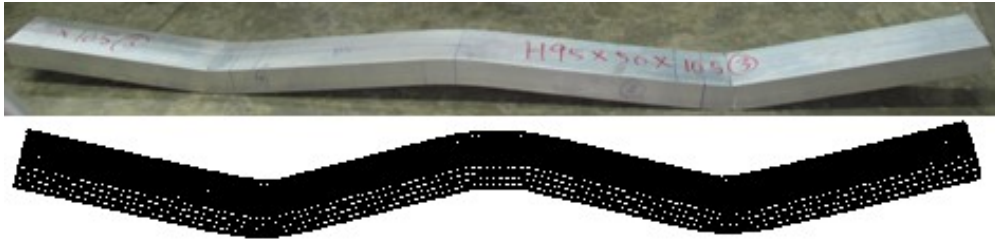
Fig. 4.6 Experimental and numerical failure modes for specimen H95×50×10.5B5I
