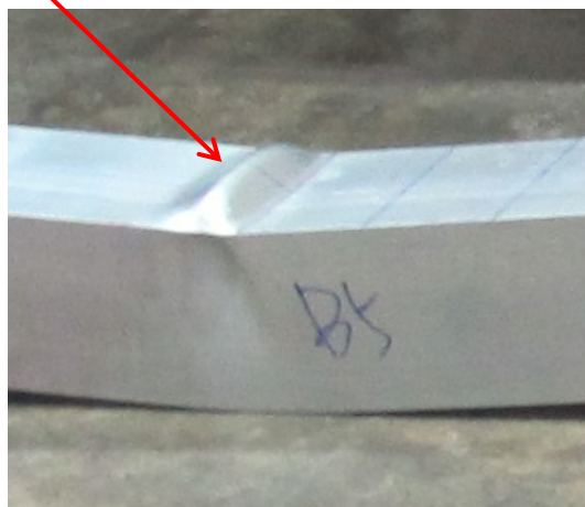
Fig. A.3.4 Inelastic local buckling on the compression flanges of five-point bending beam (H64×64×3.0B5I)
