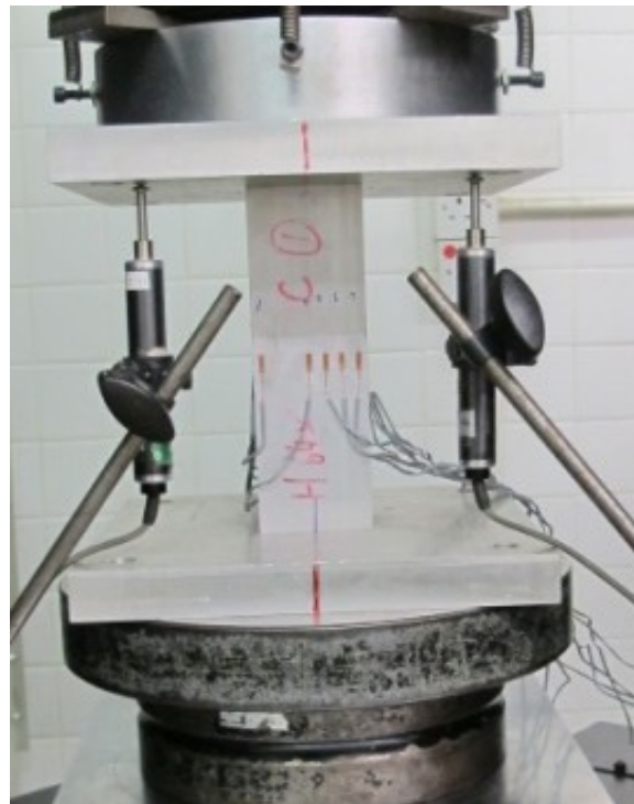
Fig. 3.10 Stub column test configuration for specimen H70×55×4.2C
