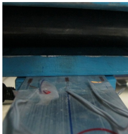
Fig. 3.16 Strain gauges attached on the compression flange
