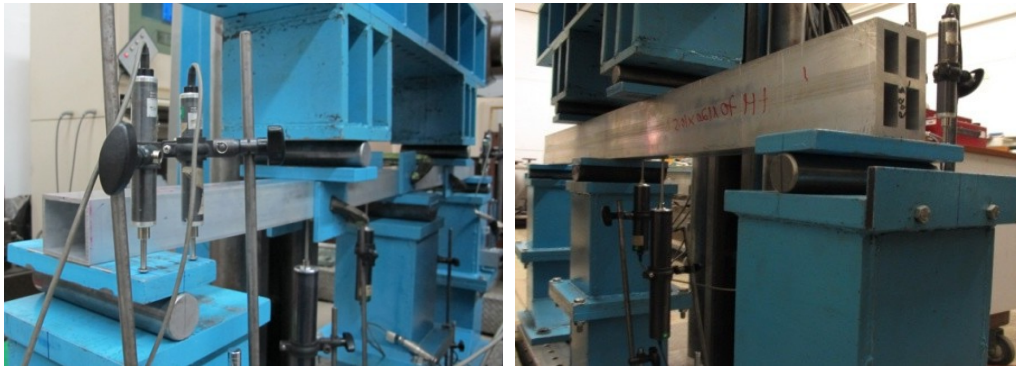
Fig. 3.24 Experimental setup for five-point bending tests
