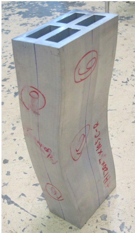
Fig. A.1.3 The attainment of global buckling on specimen (+H120×70×10.5C-R) after ultimate load
