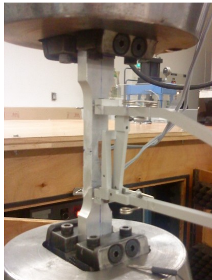
Fig. 3.5 Tensile coupon test with two strain gauges and an extensometer to measure strain
