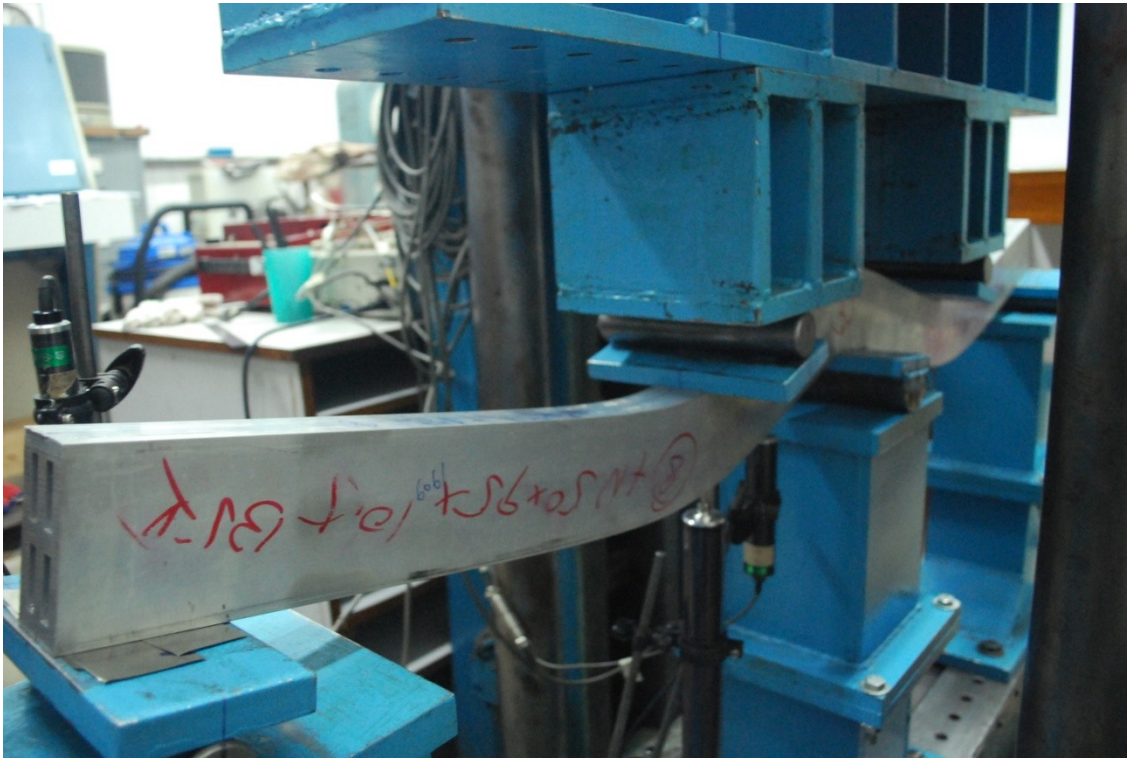
Fig. A.3.2 Large deflection of specimen (+N50×95×10.5B5II) before failure
