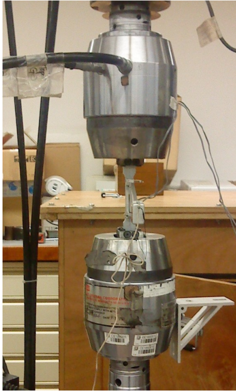
Fig. 3.4 Tensile coupon test set-up
