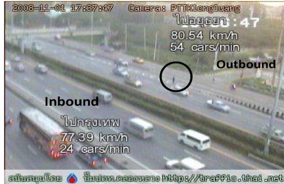
Fig. 1: Transient anomaly caused by a pedestrian on the shoulder of a freeway segment.
