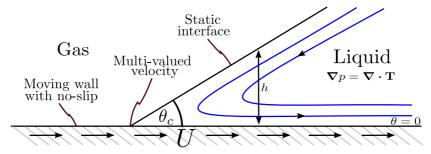
Figure 1. Model of contact line motion in a wedge geometry with contact angle  $\theta_c$ , working in a frame of reference where the contact line is stationary and the solid is moving with nondimensional velocity U.
