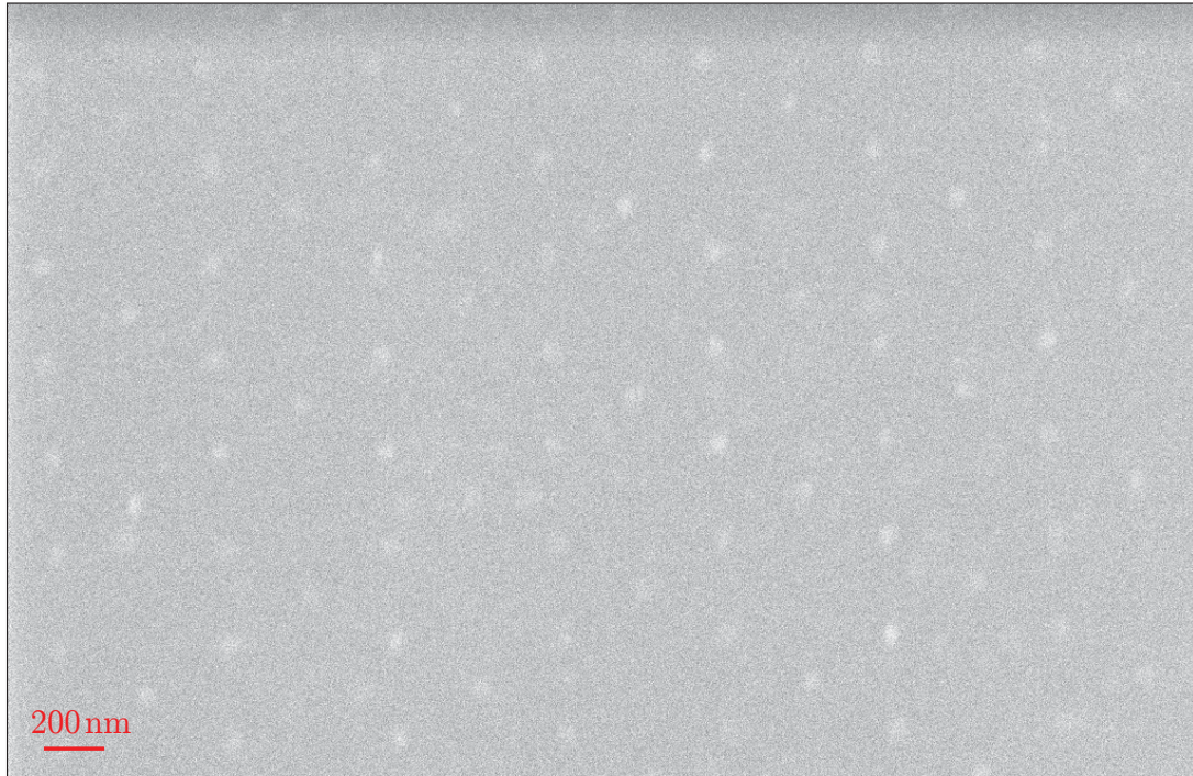
Figure 7.15: Scanning Electron Microscopy image (taken by Megha Chadha) of nanodiscs in a kagome geometry, a = 328 nm, on a silicon nitride membrane at a magnification of 28000.
