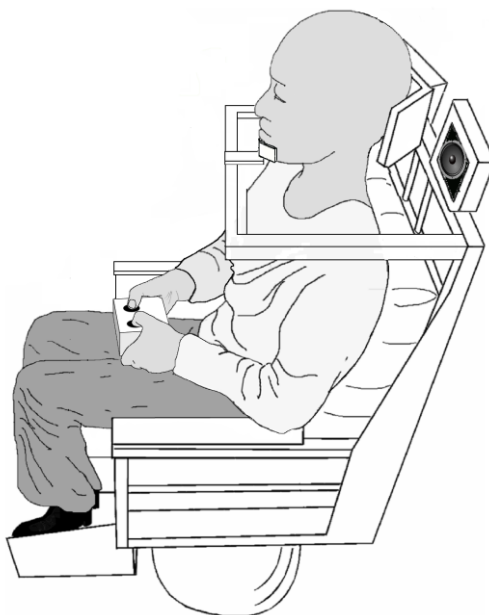
Figure 2.1. Left and Right push buttons to indicate 1 st and 2 nd interval forced responses, respectively. Chin and head rests maintain head ear canal orientation. Loudspeakers provide white noise.
