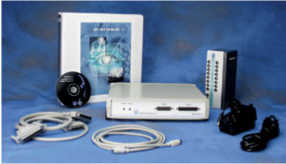
Figure 23 -Biopac MP100 and AcqKnowledge ECG system.
