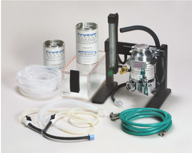
Figure 11- Bench top small mammal anaesthesia set up as provided by Vetequip.
