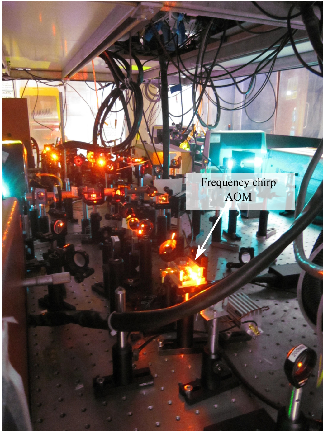
FIGURE E.2: The frequency-chirp AOM. All laser cooling frequencies from the \nu_{00} and \nu_{10} lasers are combined and double-passed through a broad-band AOM with starting frequency of 225 MHz.
