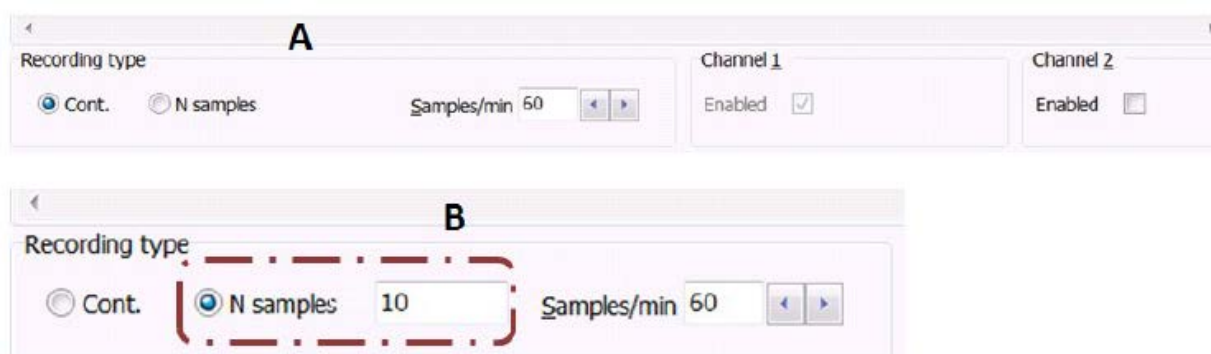
Fig. E.2.8 (A) Selecting recording type mode, (B) Recording in N-sample mode.
