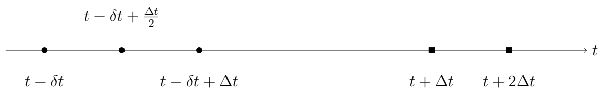
Figure 2.18: Assume that we are on the, say, even timeline with whole \Delta t increments, then the timeline with \frac{1}{2}\Delta t will be the odd timeline. If we want to calculate t + 2\Delta t from t + \Delta t , then we require historical values (with a \delta t shift) on the timelines of t + \Delta t which are t - \delta (from even timeline), t - \delta t + \frac{\Delta t}{2} (from odd timeline) and t - \delta t + \Delta t (from even timeline). This bias causes the errors accumulate unevenly and therefore the system will desynchronise.
