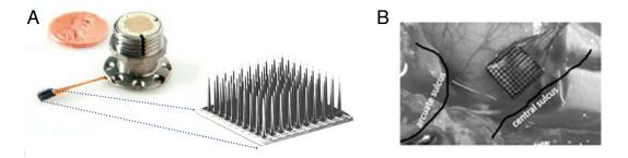
Figure 4. Blackrock microelectrode array used for intracortical recordings of neuronal activity. A: Implant and the scull interface shown next to one United States penny coin for scale. B: Example of implanted Blackrock array. Figure taken from brochure for Blackrock Microsystems<sup>TM</sup>.
