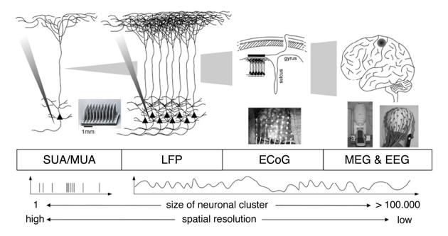
Figure 3. Overview of recording techniques used to achieve BMI control. Microelectrode arrays are used to record activity from multiple single neurons (SUA, MUA) and local field potentials (LFP). Electrocorticography (ECoG) records electrical potentials from the surface of the brain. Non-invasive recording techniques, such as MEG and EEG, record neuronal activity outside of subject's skull. Figure taken from (Waldert et al., 2009).
