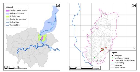
Figure 2: Cranbrook catchment (a) general location; (b) sensor location, sewer network and radar grid over the catchment.
