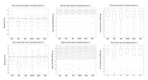
Figure 8: Boxplots of *RE* (left), *NSE* (middle) and *R* (right) for flow depths and rates simulated using different rainfall inputs for Portobello's Storm 1. The shaded areas in the *NSE* boxplots correspond to the region of positive *NSE* values (0 < *NSE* <1).
