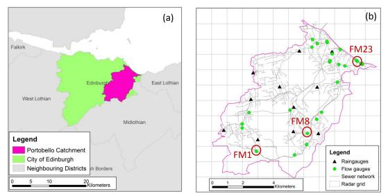
Figure 3: Portobello catchment (a) general location; (b) sensor location, sewer network and radar grid over the catchment.
