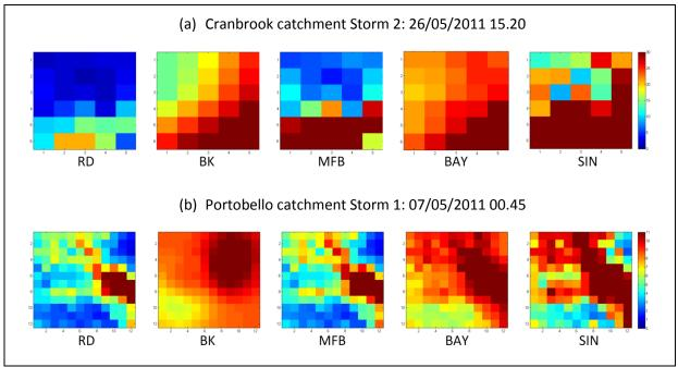
Figure 4: Images of RD, BK and adjusted rainfall estimates at peak intensity times of (a) Cranbrook's Storm 2 and (b) Portobello's Storm 1.
