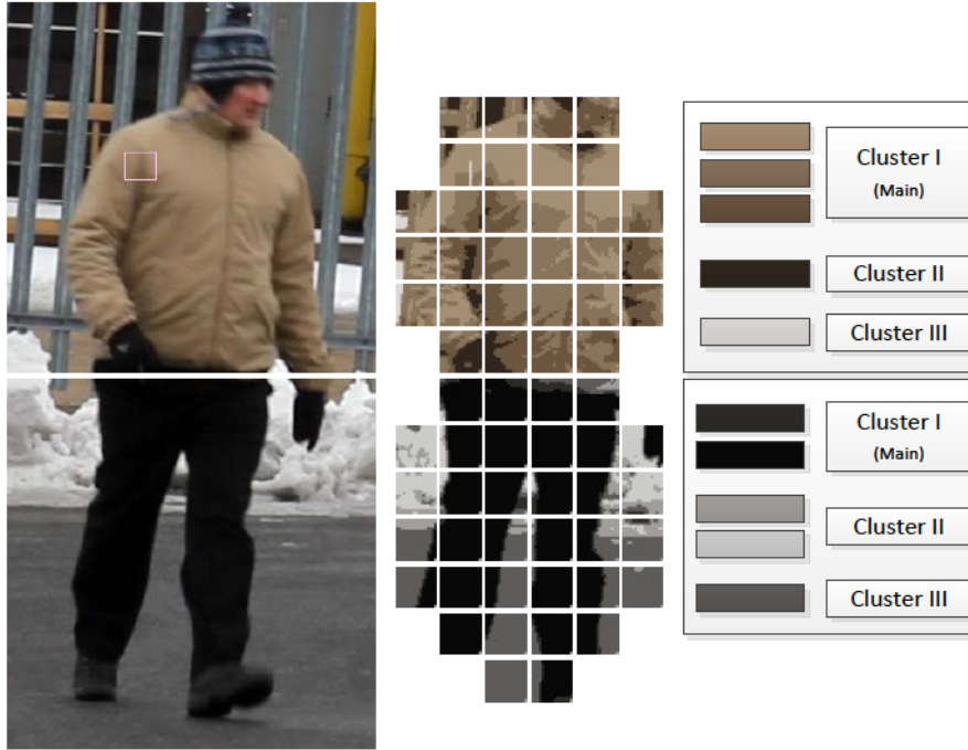
Fig. 3.4 The result of the clustering of pixels within the rough area of upper-body and lower-body of a prototype wearing mono-coloured top and bottom.
